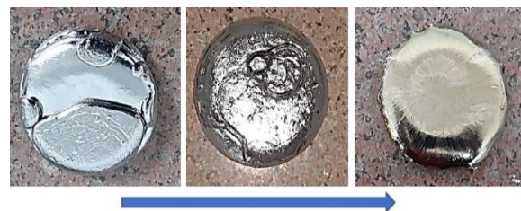
Fig. 10 Homogenization of an arc melted sample by repeating the melting process.
