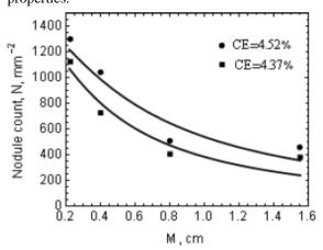
Fig. 4 Nodule count for different values of carbon equivalent (CE), CE = C + 0.33Si [8].
