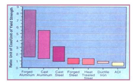
Fig. 2 Costs of different materials for obtaining unit of yield strength [7].
