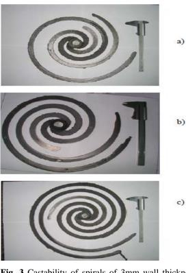
**Fig. 3** Castability of spirals of 3mm wall thickness poured into mold with different molding materials: classical a), SHMS b) and SHMS with LDASC c) [12].
