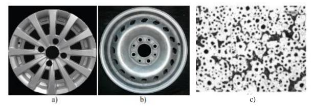
**Fig. 11** Wheel rim produced from Al-Si7Mg alloy – a), wheel rim produced from DI - b) and microstructure of thin wall ductile iron in wheel rim (2mm) - c) [8].
