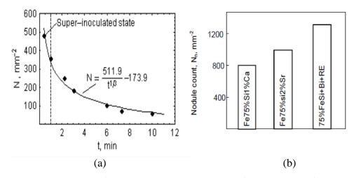
Fig. 5 Nodule count versus time after inoculation (a) and nodule count for various types of inoculants (b) [8]
