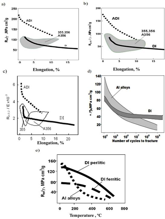
**Fig. 1** a) Tensile strength, b) yield strength, c) stiffness, d) fatigue strength and e) high temperature strength [2].
