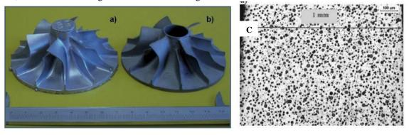
Fig. 8 Rotors: (a) aluminum alloy, (b) TWCI and (c) structure of rotor vane with 1.0 mm wall thickness [2].
