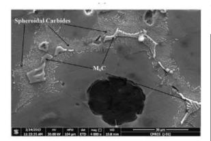
**Fig. 7** Microstructure of SiMo ductile iron, showing graphite nodule in ferrite (white) with carbides of  $M_6C$ -type (M=Fe, Mo, Si), formed in the intercellular regions.
