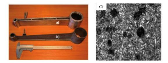
**Fig. 10** Cantilevers made from: (a) Al- alloy (weight 580 g), (b) TWADI (weight 380g) and (c) microstructure after heat treatment [2].
