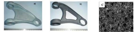
**Fig. 9** Control arms made from: (a) forged Al- alloy (weight 585 g), (b) TWCI (weight 480 g) and (c) microstructure after heat treatment [2].
