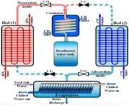
Fig.3: Schematic of adsorption desalination unit
