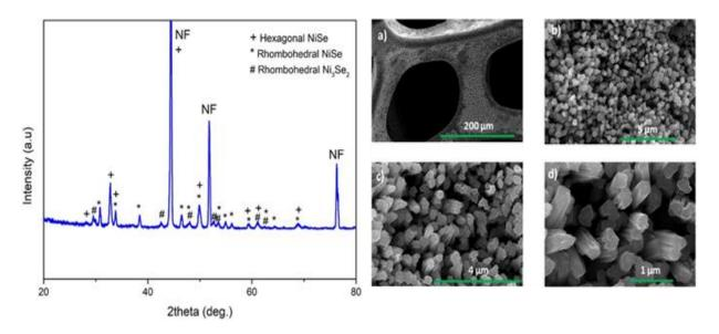
Fig. 1. XRD pattern and FE-SEM image of Ni<sub>x</sub>Se<sub>y</sub> nanorod array.
