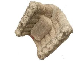
Fig. 1. Investment mold containing six tensile and impact specimens
