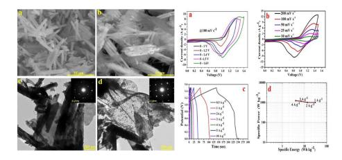
Fig. 3. SEM and TEM image and SC electrochemical performance of SnSe/rGO
