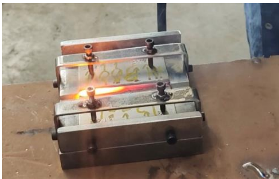
Fig. 1 Designed fixture to hold the samples during the welding process
