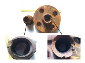
Fig. 1 Fracture surface off the flange and connected pipe (as received).
