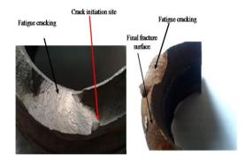
**Fig. 3** Close-up views of the fractured section of the flange depicting the fracture initiation zone, the fatigue fracture or beach zone, and the final fracture surface.
