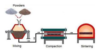
Fig. 9 The flow diagram in PSM production of parts.
