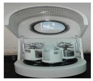
Fig. 6 Four Vails Mechanical Mixer.
