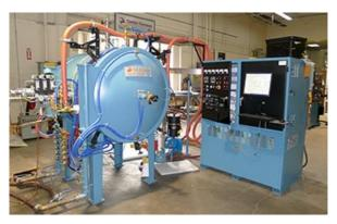
Fig. 8 Vacuum Sintering Furnace
