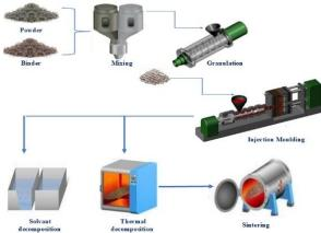
Fig. 10 Powder injection molding steps [19].
