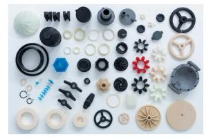
**Fig. 14** Spare parts by additive manufacturing technique [37].
