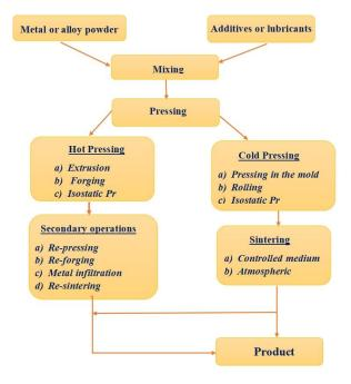
Fig. 5 Flow chart of the conventional PM process.
