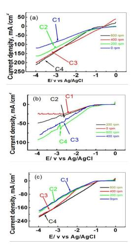
**Fig. 3** LSV curves obtained on a) Pt electrodes, b) on SS electrodes and c) on Cu electrodes in non- aqueous solution of CoFe<sub>2</sub> alloy, scan rate  $(10 \text{ mVs}^{-1})$  at different speed of stirring.
