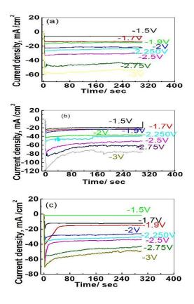
**Fig. 7** Variation of current density with time at constant potential for  $CoFe_2$  alloy on a) Pt, b) SS and c) Cu substrates from alcoholic medium.
