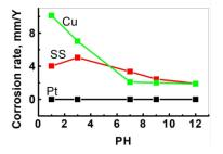
**Fig. 12** Corrosion rate versus pH curve for cobalt ferrite from non-aqueous medium) on (Pt, SS, Cu) substrates in different pH solutions.
