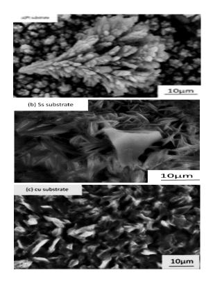
Fig. 15 SEM images of  $CoFe_2O_4$  Ferrites electrodeposited from non-aqueous sulphate bath on (a-Pt, b-SS and c-Cu) substrates.
