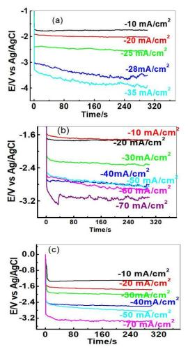
**Fig. 5** Variation of deposition potential with time at constant current density for  $CoFe_2$  on a) Pt, b) SS and c) Cu electrodes from alcoholic bath.
