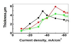
Fig. 8 Variation of film thickness with current density for  $CoFe_2$  alloy on (a- Pt, b- SS, c- Cu ) electrodes from alcoholic medium.
