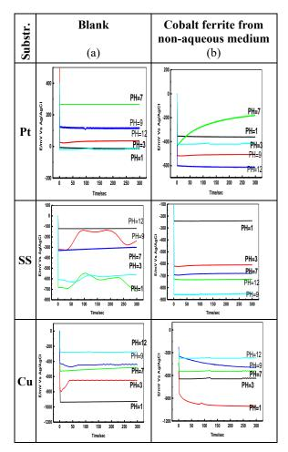
**Fig. 9** Potential-time curves of cobalt ferrite from (a) blank, (b) alcoholic medium on (Pt, SS, Cu) substrates in different pH solutions.
