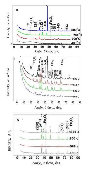
Fig. 13 XRD patterns of  $CoFe_2O_4$  Ferrites electrodeposited from non-aqueous sulphate bath on a-Pt, b-SS, c- Cu substrates.
