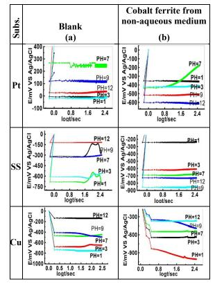
**Fig. 10** Potential-log t curves for cobalt ferrite from ablank, b- non-aqueous medium) on (Pt, SS, Cu) substrates) in different pH solutions.
