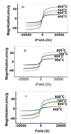
Fig. 14 Effect of annealing temperature on M-H hysteresis loop of  $CoFe_2O_4$  annealed at 400, 600, 700 and 800 °C.
