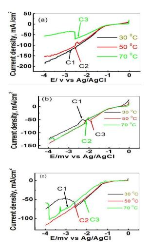
**Fig. 4** LSV curves obtained on a) Pt electrode, b) SS electrode and c) Cu electrode in non-aqueous solution. of CoFe<sub>2</sub> alloy, scan rate (10 mVs<sup>-1</sup>), at different temperatures.
