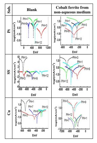
**Fig. 11** Tafel plots polarization curves for cobalt ferrite from for a) aqueous medium, b) alcoholic medium) on (Pt, SS, Cu) substrates in different pH solutions.
