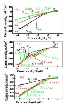
**Fig.2** Voltammograms obtained on different substrates in non-aqueous solution of a)  $0.05 \text{ M CoSO}_4$ ; b) 0.1 MFe (NH<sub>4</sub>)<sub>2</sub>(SO<sub>4</sub>)<sub>2</sub>, c- CoFe<sub>2</sub> alloy, and solution of CoFe<sub>2</sub> alloy at SR (10 mV/s) and 0 rpm.
