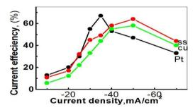
**Fig. 6** Variation of current efficiency with current density for a CoFe<sub>2</sub> alloy on Pt, SS, Cu substrates from non-aqueous bath.
