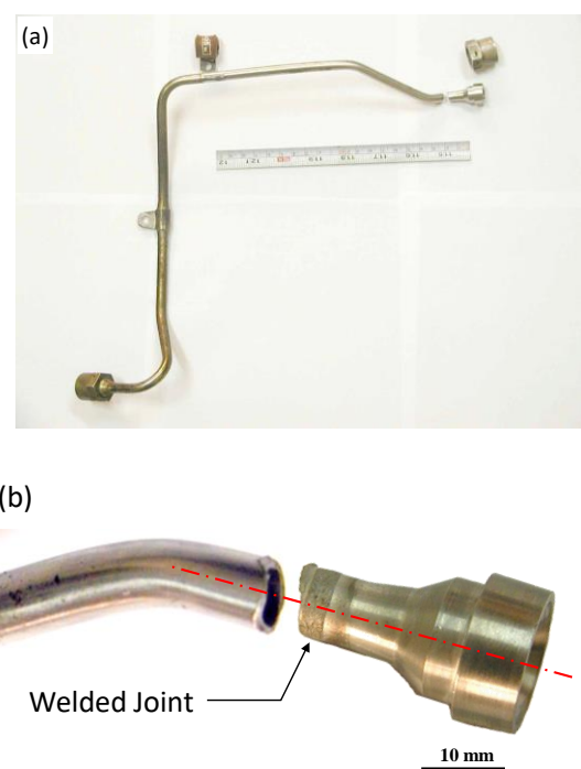
Fig. 6 (a) A general view of the fractured fuel supply tube, and (b) a close-up of the fracture zone.
