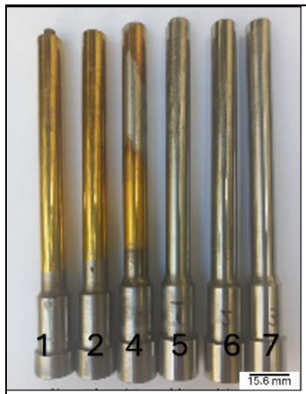
Fig. 3 (1) original punch, (2) original failed punch, (3) equivalent K110 punch, and (4-6) three local manufactured failed punches.
