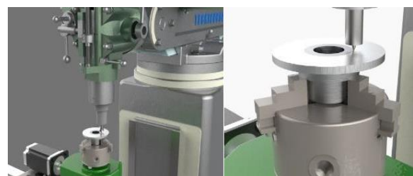
Fig. 2 The Fixture and Set Used to Induce FSW for a Flange in Schematic Form.
